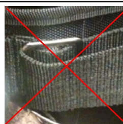
Incorrect and correct fabric buckle lacing
